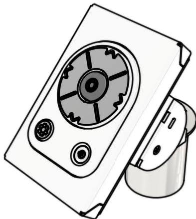
ADA-Pad installation solution for poles
