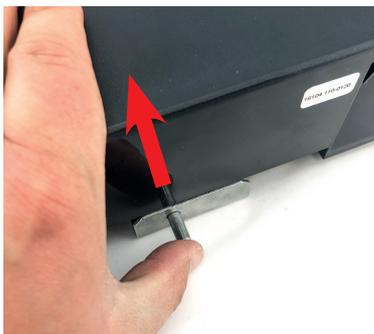
**Possibility 2:** Lightly pressing the cassette when actuating the release plunger
